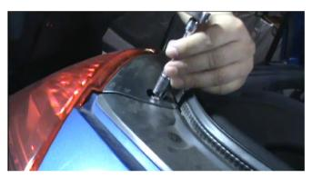
2) Once the fasteners have been removed, you will need to remove (3) 10mm nuts, shown here.
