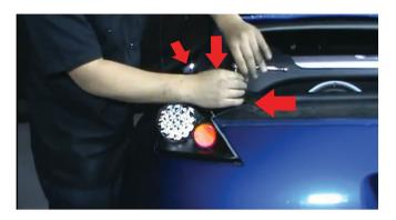
8) Finally, seat the head light back on the vehicle lining up the mounting holes with the bolt holes. Once this is done reinstall the (3) 10mm bolts and plastic fasteners. Complete these instructions for both sides.
