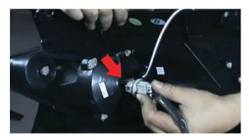
7) Now that everything is wired and connected, twist the socket from the brake harness into the tail light housing clockwise. Be sure it is seated properly to prevent any condensation in the tail lights.
