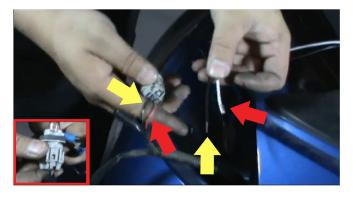
4) Shown here is the running light harness from the vehicle and the LED running light wires from the Spyder lights. You will need to spice these wires together, Black with black and white with red. Note: you can identify the running light by the bulb sizing, running light will be the smaller bulb of the two shown.
