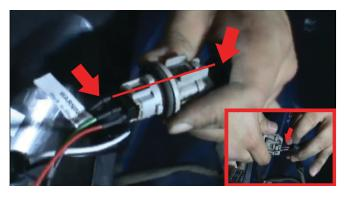
6) Next, once the brake bulb has been removed you can now insert the clip from the Spyder tail light into the brake bulb socket. Be sure you are lining up the black ground wires of both sides, installing this incorrectly can damage the harness, LED's and fuses.
