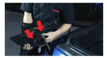
3) Next, gently push outwards from the back of the tail light to get it free. Still attached will be the tail light harness (arrows). With moderate force, twist the socket counter clockwise to unlatch it from the tail light. set OEM assembly aside.
