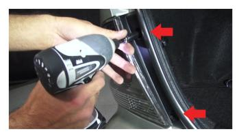
1) Open your trunk and locate the (2) 10mm bolts that hold the taillight in place. Using the 10mm socket, remove these bolts.
