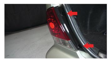
6) Final step, reseat the tail light lining the plastic pin on the back of the tail light with the mount hole on the vehicle frame. The mounting holes should line up with the bolt holes. Replace the (2) 10mm bolts to secure the tail light in place and you are done.
