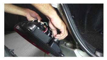
5) Next, simply insert the sockets in to the tail light housing, placing the bulbs in there designated housings. Twist the sockets to secure them in place.
