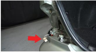
3) Next, locate the brake light bulb and gently pull it out of its socket. You can keep this bulb with your old tail lights if ever needed again.
