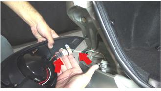
4) Shown here you will need to connect the new LED clip into the bulb socket of your vehicles tail light harness. Be sure to line up the Black ground wires from the LED clip with the White and Black wire from the vehicles harness to prevent from blowing any fuses.
