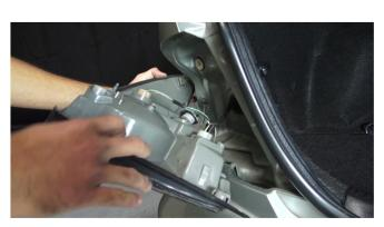
2) Once the bolts have been removed, you can remove the tail light. Once you have the wiring harness exposed, twist the 3 bulbs and sockets from the tail light.
