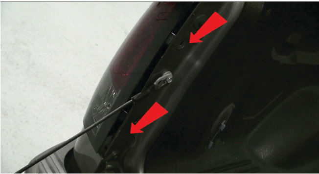
7) Reinstall the two phillips head screws that secure the tail lights.
