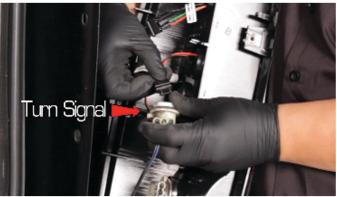
6) Install the center-position socket insert into the turn signal socket. Align the black wire side of the insert with the black wire side of the socket to ensure correct polarity. Then reinstall the turn signal socket into the center position of the Spyder tail light.
