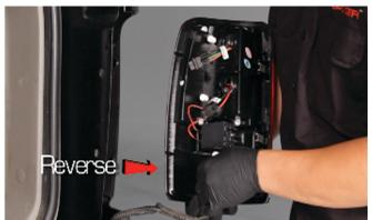
5) Reinstall the reverse lamp socket into the bottom position of the Spyder tail light.
