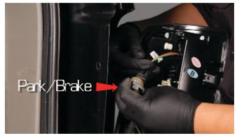
7) Install the top position socket insert into the park/brake lamp socket. Then reinstall the park/brake lamp socket into the top position of the Spyder tail light.
