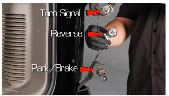
4) Remove the bulb sockets from the OEM tail light. Remove the turn signal and park/brake lamp bulbs from their sockets. Never touch exposed bulbs with bare hands.
