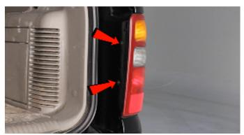
2) Remove [2x] phillips screws securing the tail light.
