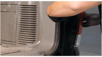
9) Reinstall [2x] phillips screws to secure the tail light.
