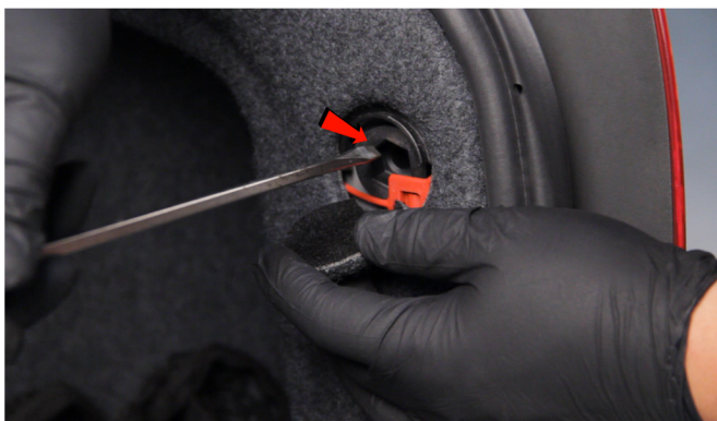
3) Use a long flathead screwdriver to remove the outer tail light screw.
