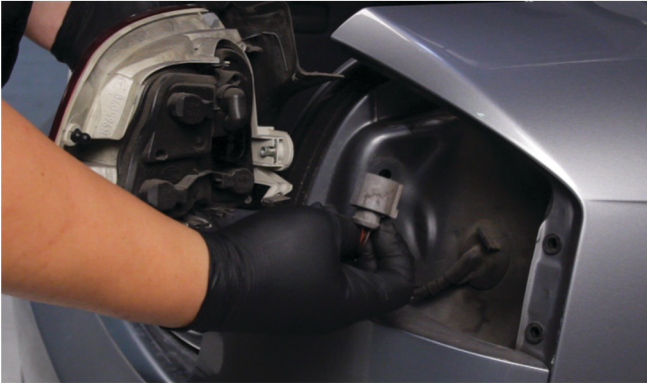
5) Disconnect the outer tail light wiring harness, then remove the outer tail light and set it aside.
