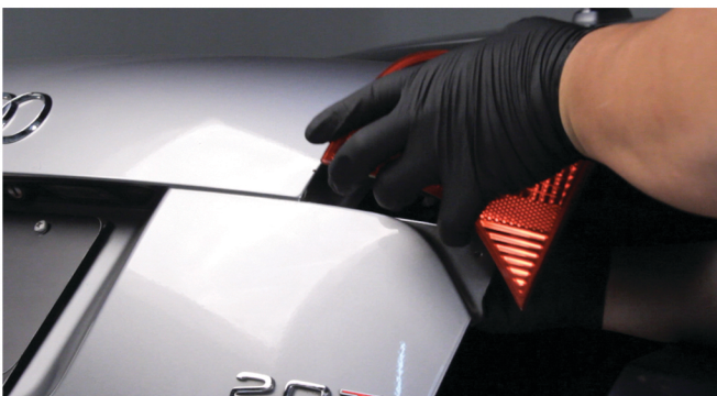
9) Unseat and remove the inner tail light.
