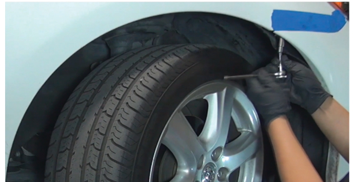
22) Reinstall [1x] 10mm bolt at the corner of the fascia to secure it.
