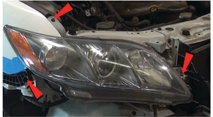
8) Remove [3x] 10mm bolts securing the headlight.
