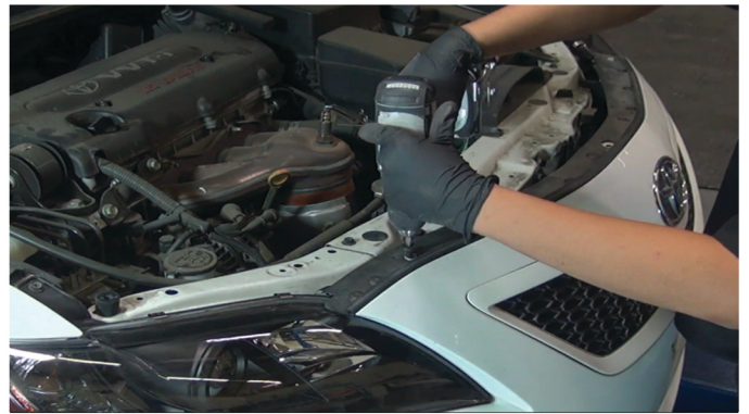
20) Reinstall [2x] phillips screws to secure the fascia.
