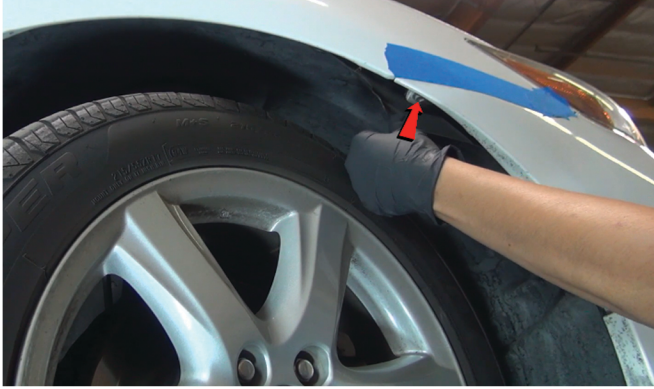
5) Remove [1x] 10mm bolt securing the fascia to the fender.
