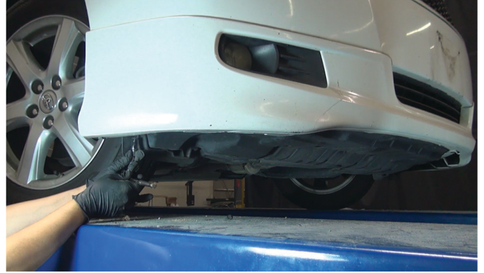
24) Reinstall [6x] 10mm bolts to secure the fascia to the undertray.
