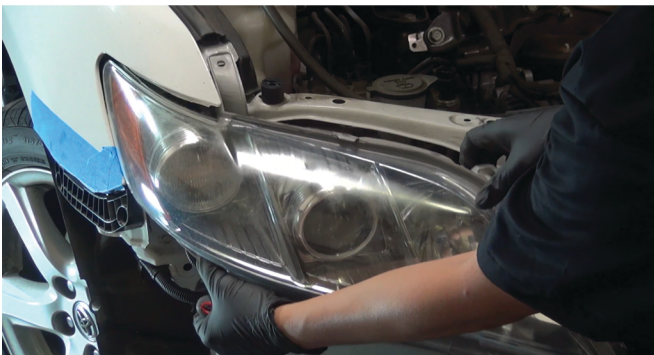
9) Release the mounting tabs to unseat the headlight.
