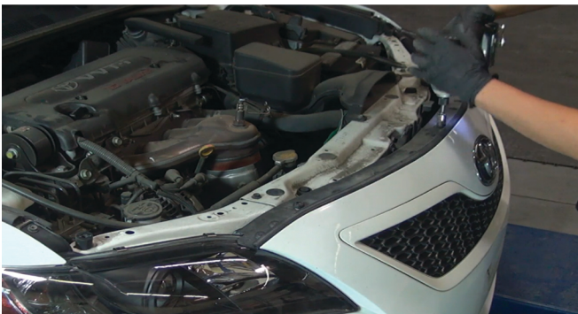
21) Reinstall [1x] 10mm bolt to secure the fascia.
