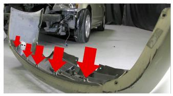
4) Remove [5x] Plastic Retainers securing bumper fascia to body. (Bumper removed for illustration purposes)
