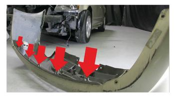
15) Reinstall [5x] Plastic Retainers securing under side of bumper fascia to the body. (Bumper shown removed for illustration purposes)
