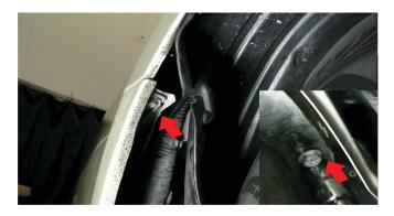
13) Move to the wheel well. Reinstall [1x] Phillips Head Screw and [1x] 10mm bolt securing bumper fascia to fender.
