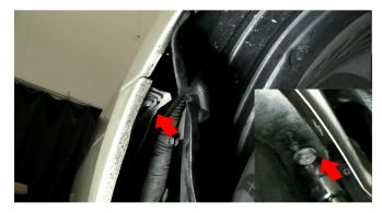
2) Move to the wheel well. Remove [1x] Phillips Head Screw & [1x] 10mm Bolt securing the fender to the bumper fascia.
