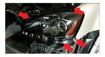
11) Install [4x] 10mm Bolts to mount and secure SPYDER headlight.
