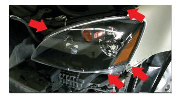
7) Remove [4x] 10mm Bolts securing headlight.
