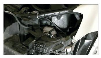
9) Disconnet the headlight by removing all bulb sockets from the OEM headlight, then remove the OEM headlight assembly and set it aside.
