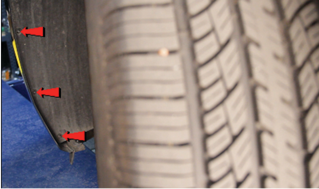
5) Remove [3x] T-15 Torx screws that secure the fender liner to the fascia.
