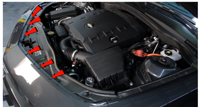
2) Remove [6x] plastic retainers securing the fascia.
