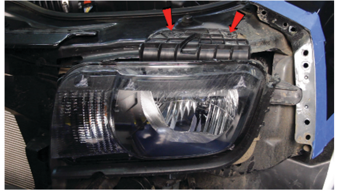
12) Remove [2x] 7mm bolts that secure the headlight from above.
