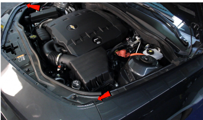
3) Remove [2x] 10mm bolts securing the fascia at the fender edge.
