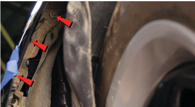
33) Reinstall [3x] 10mm bolts that secure the fascia to the fender from inside.
