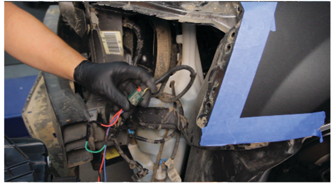
26) Reconnect the headlight wiring harness.
