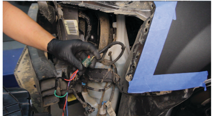
20) Reconnect the headlight wiring harness.
