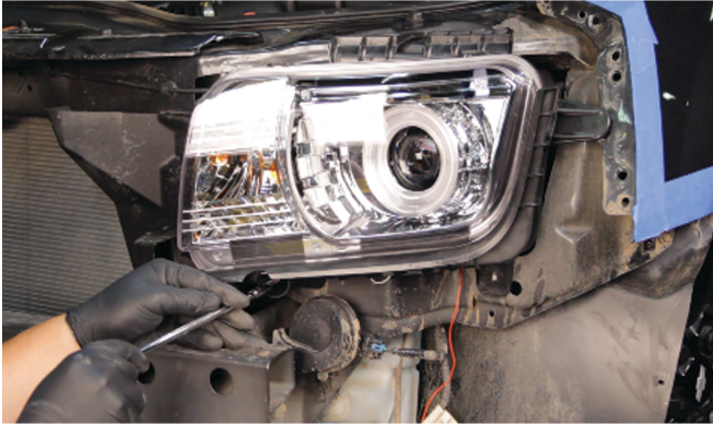
29) Reinstall [2x] 7mm bolts to secure the headlight.
