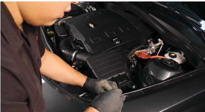
39) Reinstall [2x] 10mm bolts that that secure the fascia to the fenders.
