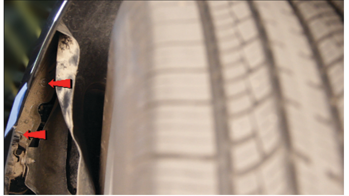
6) Remove [2x] 10mm Bolts that secure the fascia to the fender from inside the fender.
