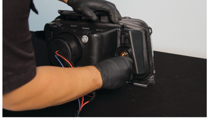
24) Reinstall [3x] 10mm bolts to mount the headlight.
