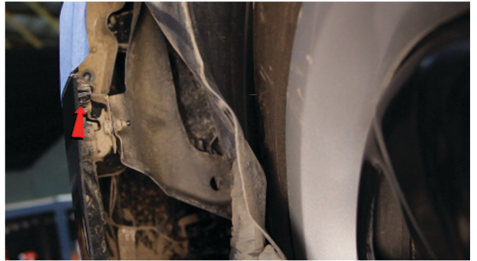
8) Remove [1x] 7mm bolt that secures the fascia to the fender.
