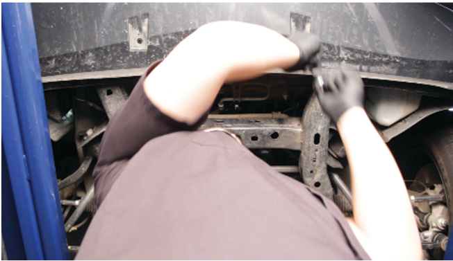
37) Reinstall [2x] 10mm bolts to secure the fascia to the undertray.
