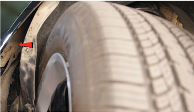
7) Remove [1x] 10mm bolt at the top that secures the fascia to the fender.
