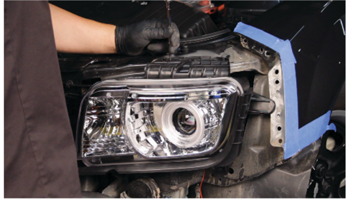
30) Reinstall [2x] 7mm bolts to mount the headlight.
