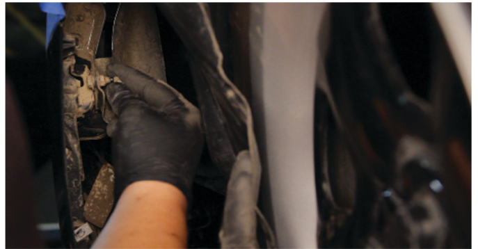
34) Reinstall [1x] 10mm bolt to secure the fascia to the fender.
