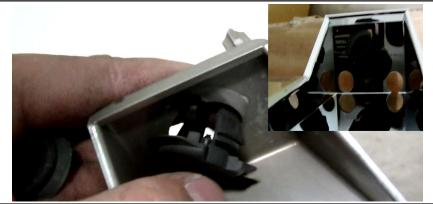
Place the grille back into place like the factory grille and lock the snap that holds the grille in place.
