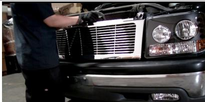
To light up the L.E.D.'s, use a quick connect and connect it to the parking lights.
